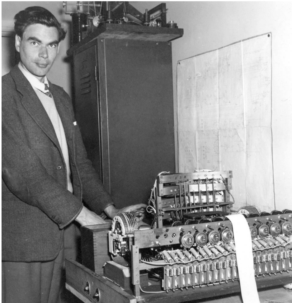
Figure 3: 'The recording device shown in the photograph, which I called Thoth, after the Egyptian god of writing and wisdom, was built to record the results (which were signalled with electrical contacts on the escape controls) of the simulation of a disabled submarine. It was based on a pallenotype machine, with a keyboard and the letters of the alphabet – used for shorthand. In front of the curved strips (below the vertical push rods) was the keyboard working the pallenotype. Unlike a typewriter any number of keys could be pressed at once. To the left is a clock, in the box, which was used by RAF fighter command for allocating add hyphen, to read: 15-second periods for transmission and reception with four different “coloured” squadrons sending pulses to the uni-selector – which is the curved object in front of the box. This part was from telephone exchanges - we used whatever we could get hold of – and was wired up to code letter keys to indicate time, I think to the nearest second. The experiment lasted ten hours. Later I redesigned the time system using a mechanical counter like the mileometer on a car, with the typeface on the wheels, which printed time in numbers. This was quicker to read. The device was then made a lot smaller and neater, later manufactured by the Cambridge Instrument Company. It was not a total success as it was not entirely reliable, but it was a start towards automatic recording.' Professor Richard Gregory, 3 and 5 December 2002.
