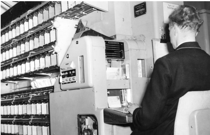
Figure 16: In the early 1960s mechanization of letter-sorting envisaged a keyboard operator copying postcodes to enable mail to be sorted electronically, as illustrated above. I was engaged by the Post Office in research concerned with alphanumeric keyboards. Dr R. Conrad, 10 February 2003.
